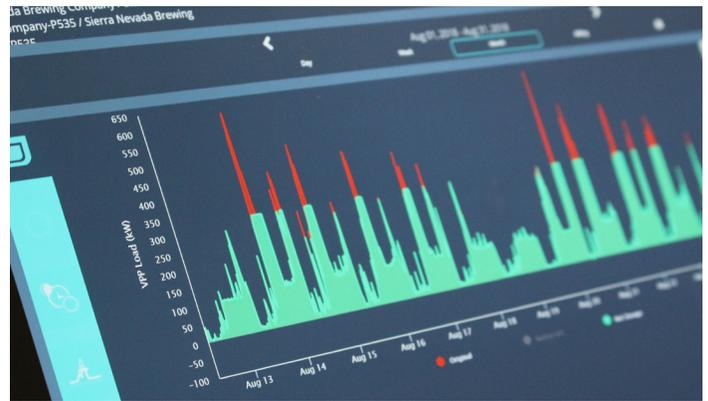
The GridSynergy cloud-based software draws on historical energy usage data as well as real-time input from the batteries on site, to calculate optimal charge and discharge cycles.
